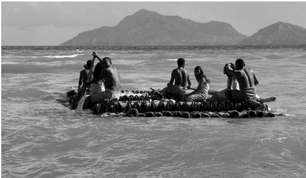
Figure 3. Stone-tool-built bamboo raft off the coast of Flores, Indonesia. This is the eighth experiment undertaken to examine how successful colonising sea crossings of the Lower Palaeolithic may have been accomplished in this region as well as in the Mediterranean. 13 April 2008.
